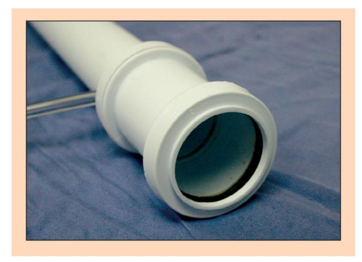
**Figure 3b.** The viewing window that when in place (as shown) has an airtight sealed allowing the effective use of air insufflation.
